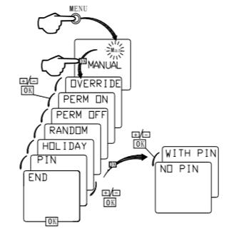
If a PIN code has been activated, the timer can no longer be activated without a valid PIN code after a RESET.
